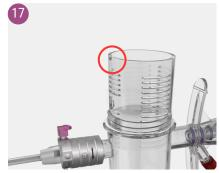
Replace the basket by positioning the notch at the top towards the quick-lock button.
