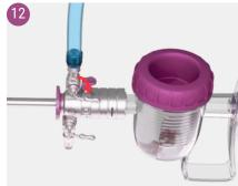
At the end of the last activation, do not wait for the cavity to fill again and close the irrigation stopcock.
