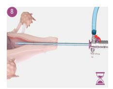
Open the irrigation stopcock and wait until the desired target pressure is obtained (minimum 100mmHg).
