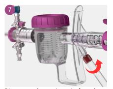
Disconnect the suction tube from the outer sheath and connect it to the back of the ICE activator.
