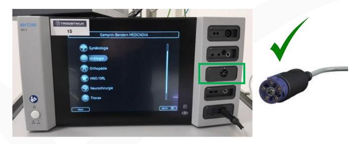
If the MF plug is not installed, use the Erbe bipolar adapter MF-2 and MF-U-socket, MF-plug on the MF-U plug
